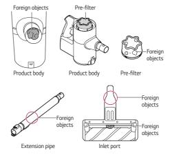
※ If the inside of the product body, extension pipe, or inlet port or the pre-filter itself is clogged with foreign objects, the power automatically turns off to protect the product. Separate the battery from the product and remove the foreign objects.
